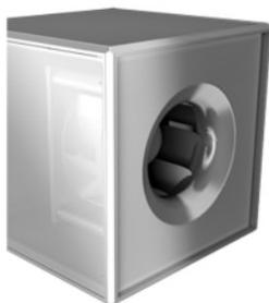
The housing supporting frames are double chamber aluminum profiles with corners made of plastic and double skinned (20mm) galvanized steel panels insulated with non-inflammable, noise and temperature insulating fiberglass mats. One side of the casing is open as standard.
