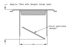
**PSTP** – Pressed steel toe plate - No. 28 Type C As PSFD & PSCD with no damper mechanism.
