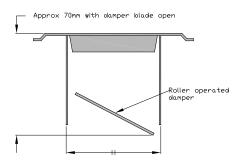
PSCD - Pressed steel ceiling diffuser - No. 28 Type B
