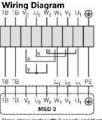
Three phase motor with 2 speeds and thermostatic switch (TB). Speed changing by  ${\rm MV}$  switching. Changing of rotation direction by interchanging of 2 phases. If MSD 2 2-step switching units are used do not insert bridge and connect dotted lines in the wiring diagram to the switching unit.
