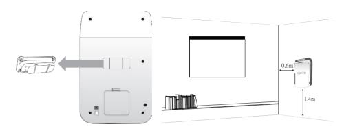
X It is recommended that the Device (bottom of device) is positioned such that it operates 140cm away from the floor and a minimum 60 cm away from the wall.
