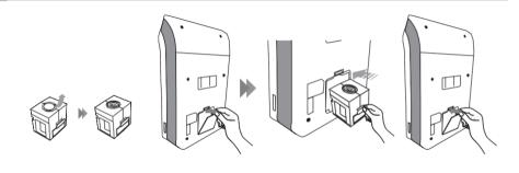
④ Hang the Device up with the wall bracket, making sure the Device locates fully with the wall bracket as indicated.
